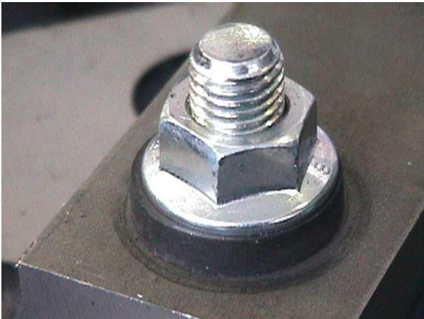
Fig. 31: correct assembly of the vibration dampers;
